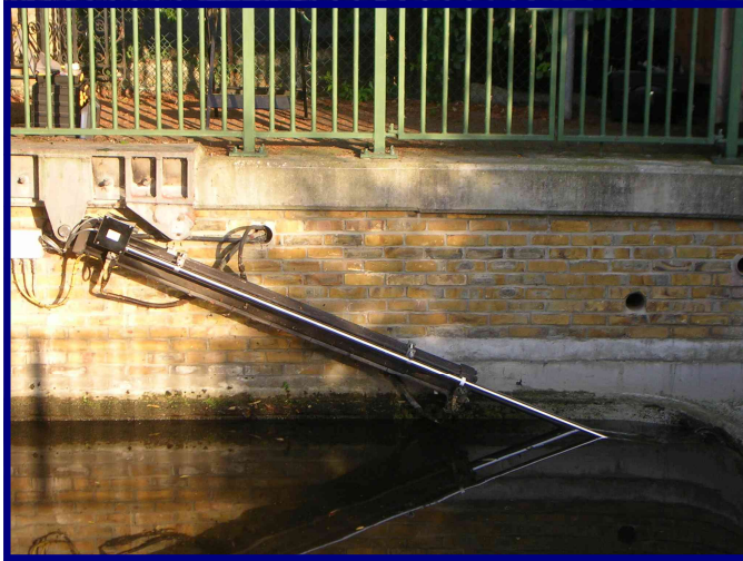
Telescopic Position Sensor Measuring Range: Up to 2 meters.
